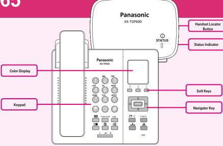
handsets KX-TGP60 can be registered to a single Base Unit KX-TGP600. To add a new desk phone or handset press and hold the location button (on the right side) on the Base unit for about 3 seconds. The STATUS indicator will flash red. On a not registered Desk phone, press and hold "OK" until "Please Wait ....." displays. After "Registered" is displayed on the LCD, the registration is completed. If the telephone is already registered to a Base station, do the
