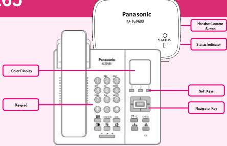
handsets KX-TGP60 can be registered to a single Base Unit KX-TGP600. To add a new desk phone or handset press and hold the location button (on the right side) on the Base unit for about 3 seconds. The STATUS indicator will flash red. On a not registered Desk phone, press and hold "OK" until "Please Wait ....." displays. After "Registered" is displayed on the LCD, the registration is completed. If the telephone is already registered to a Base station, do the
